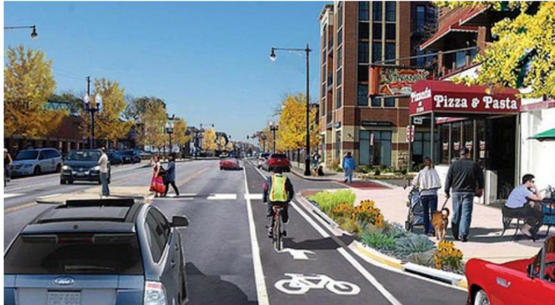
Bumpouts can be utilized to accommodate bio-infiltration as a Low Impact Development (LID) strategy for treating stormwater runoff.
