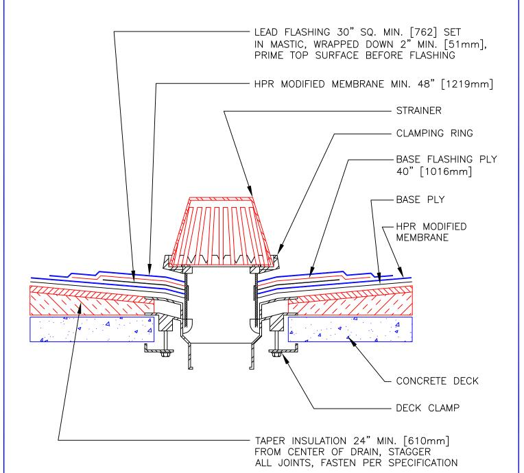
ALL PLIES SET IN MODIFIED COLD ADHESIVE SEE SPECIFICATIONS FOR SURFACING
