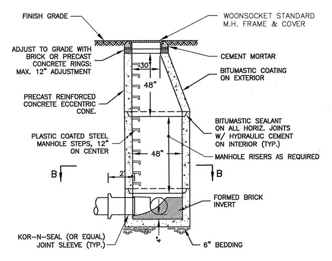
NOTE: ALL LIFTING HOLES TO BE PLUGGED IN AND OUT WITH HYDRAULIC CEMENT.
