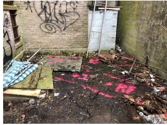
Picture 4: End of Alley. Both anomalies were found to have Radio Frequencies. The near one was seen at 1-2' deep, the farther was too close to the wall to be detected with GPR.
