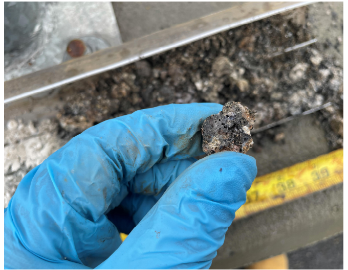
Photo depicts a clinker found within shallow soils at soil boring B-5.
