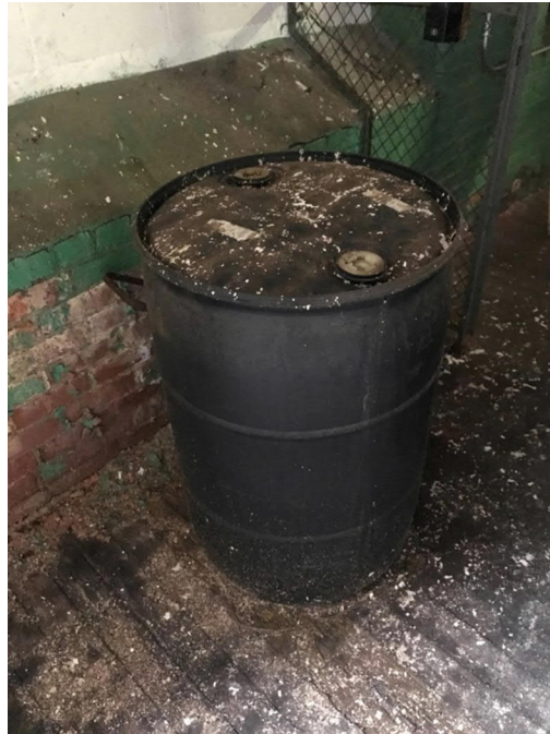
Figure 17: Slight bulging drum on the first floor.
