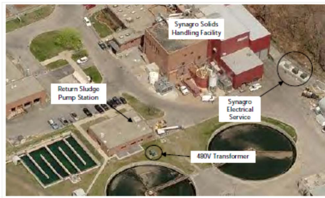
FIGURE 8-9 AERIAL VIEW OF ELECTRICAL POWER SERVICE – SOUTH END
