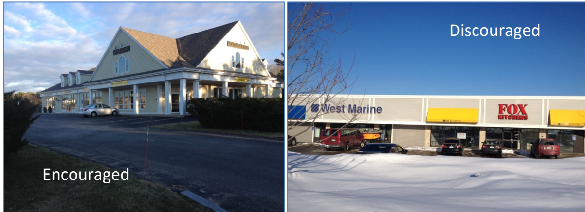
Figure 3: Peaked roof reduces the building mass on the left while the flat roof on the structure to the right not only makes a building look more expansive but does look as visually interesting.
