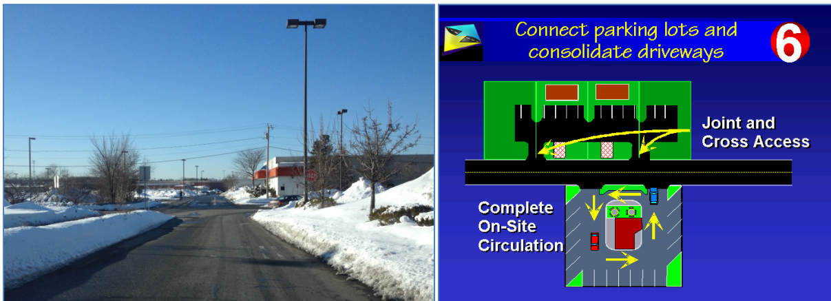
Figure 8: Interior access roads between retail developments help reduce vehicular volume and turning movements on major roadway. Image on right demonstrates how the number of curb cuts from individual properties can be reduced through joint and cross access and complete on-site circulation 2
