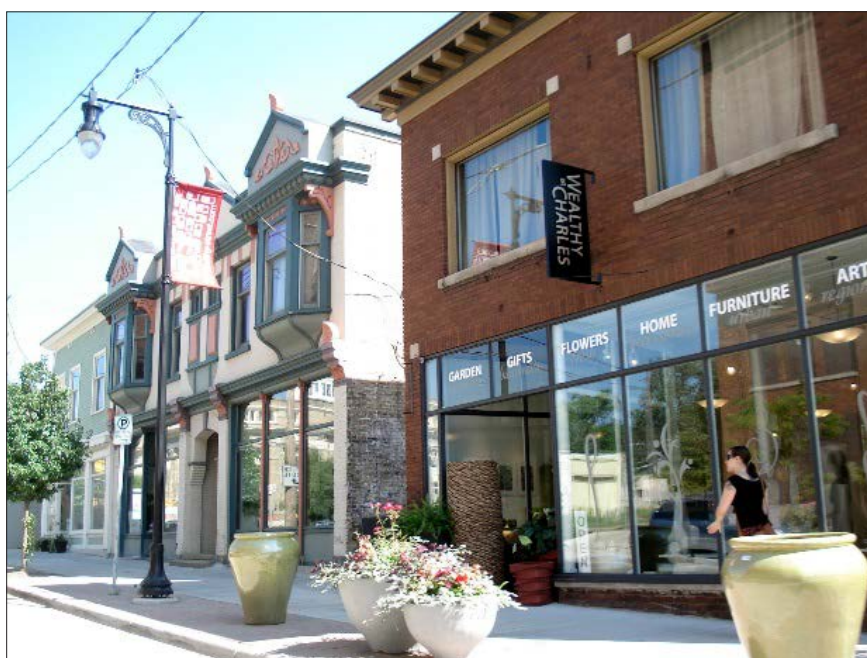
FIGURE 6. Large, clear ground-floor retail windows visually draw pedestrians inside. Transom windows further increase the light into the building.
