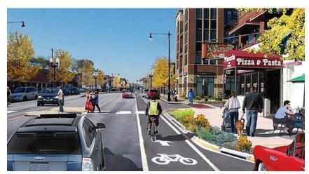
Bumpouts can be utilized to accommodate bio-infiltration as a Low Impact Development (LID) strategy for treating stormwater runnoff.
