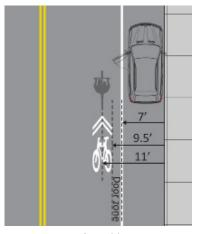
Positioning the SLM 11 feet from the curb encourages cyclists to stay clear of the door zone
