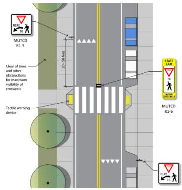
Plan view of a high-visibility crosswalk, signage and bump out
